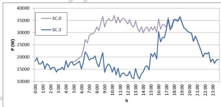
Figure 13. Comparison of the daily load profiles in SC.0 and SC.3
