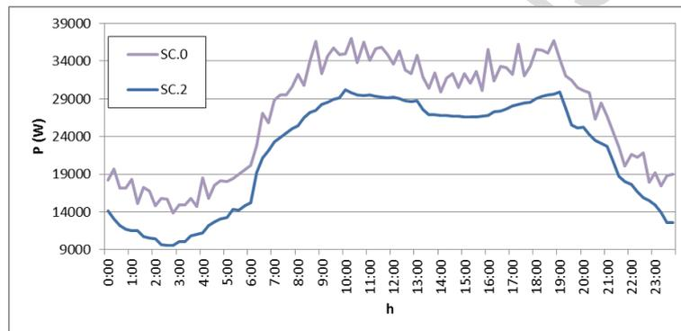
Figure 12. Comparison of the daily load profiles in SC.0 and SC.2
