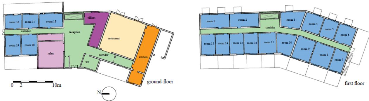
Figure 2. Plans of the hotel with thermal zone highlighted by colors.
