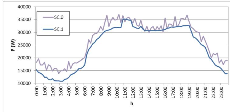
Figure 11. Comparison of the daily load profiles in SC.0 and SC.1
