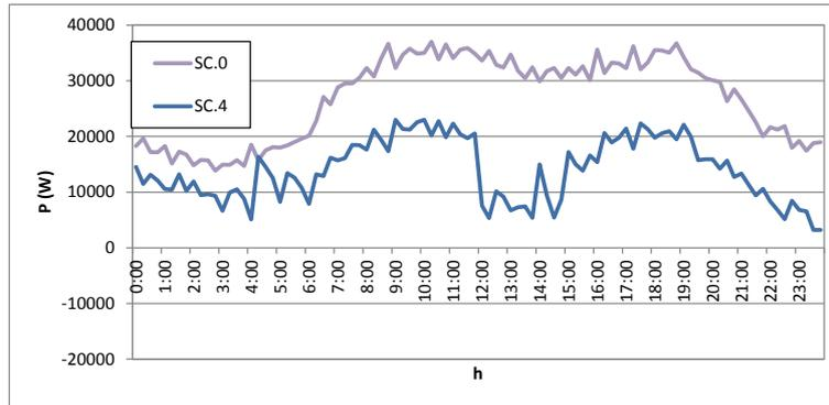
Figure 14. Comparison of the daily load profiles in SC.0 and SC.4
