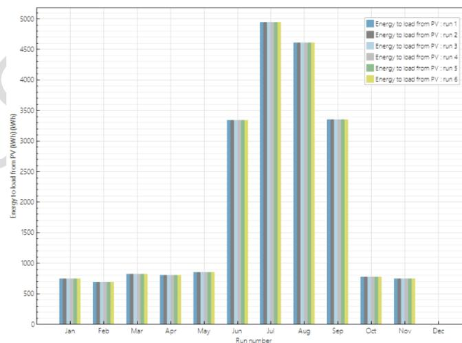
Figure 9. Monthly summary of the electricity produced by PV plant and consumed by the heat pump.
