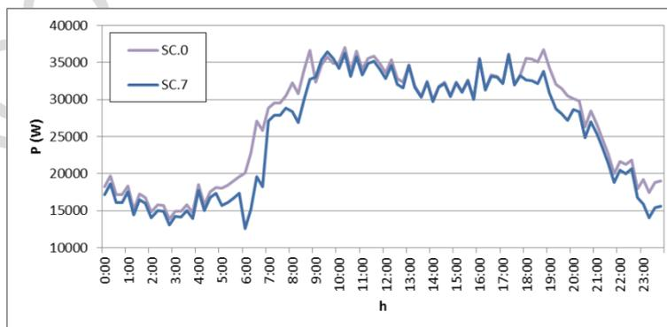
Figure 17. Comparison of the daily load profiles in SC.0 and SC.7
