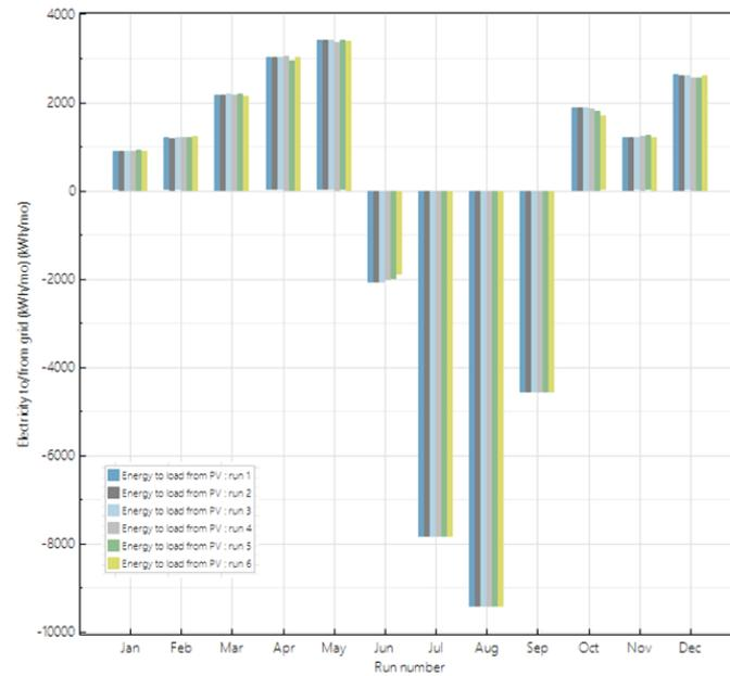
Figure 8. Monthly summary of the electricity from/to the grid.
