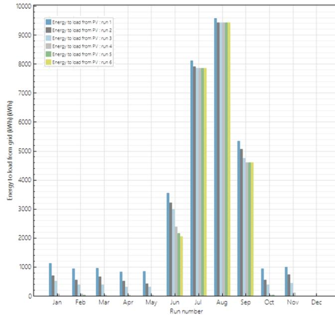
Figure 10. Monthly summary of the electricity from the grid consumed by heat pump.
