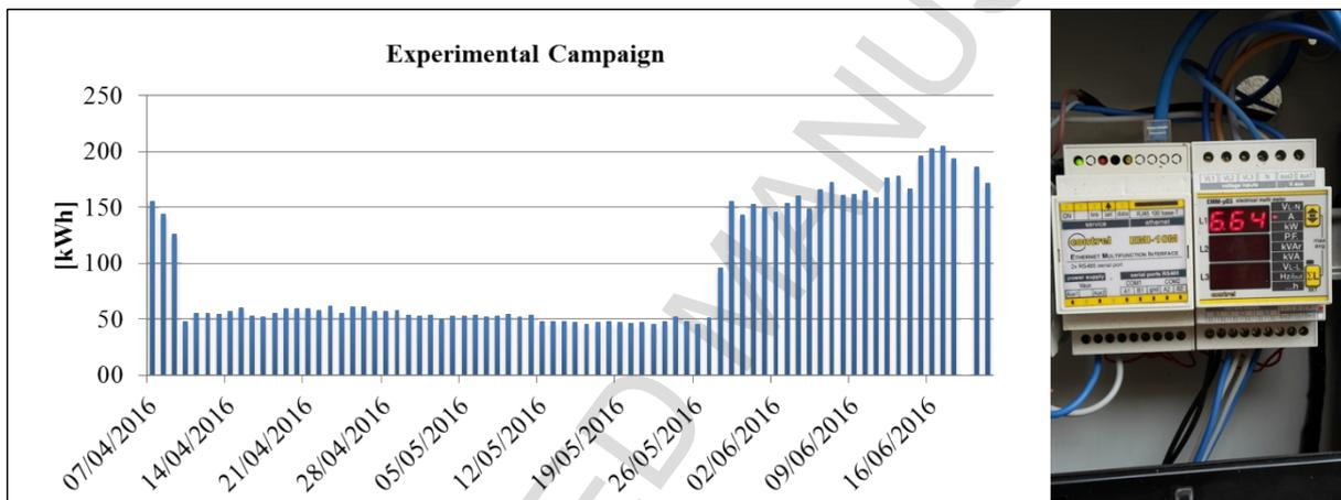
Figure 4. Electricity consumption survey and picture of the smart meter.
